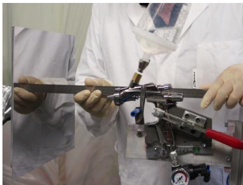
Fig. 2 : Set-up of spray gun in front of the target
