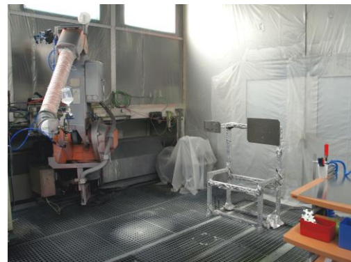
Fig. 3 : Arrangement of panel holder inside the spray booth (air humidity, temperature and downdraft velocity see individual data sheets)
