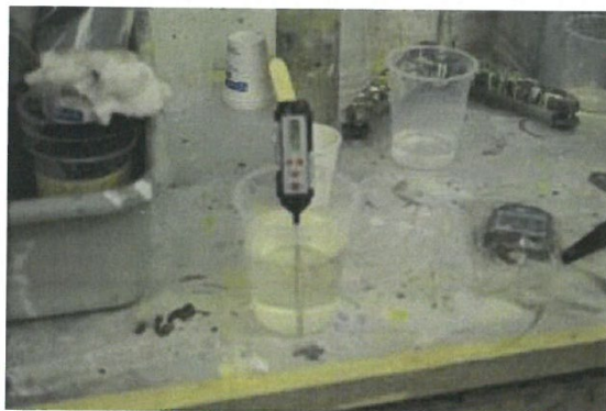
Figure 19: Clearcoat Temperature Check
