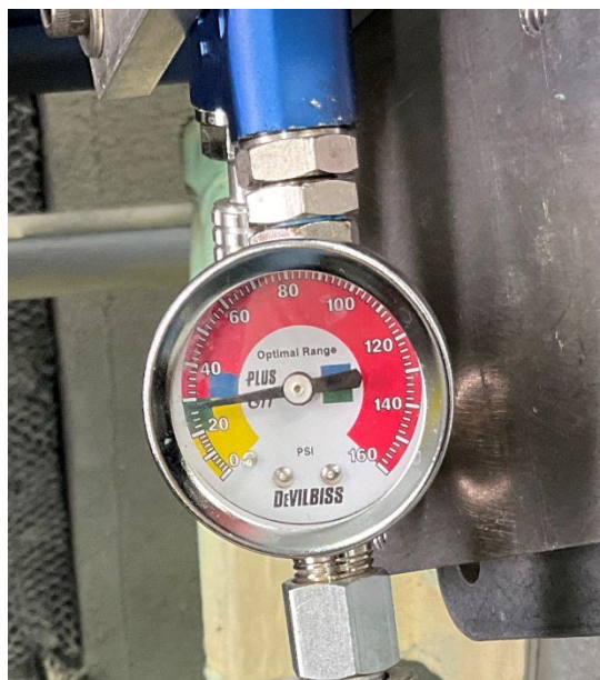
Figure 7: AI Basecoat Inlet Air Pressure Check
