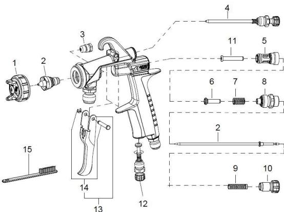
◆ Marked parts are wearable parts.
