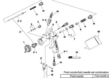
When ordering parts, specify gun's model, part name with ref. No. and marked No. of air cap set, fluid nozzle and fluid needle. Marked parts are wearable parts.
